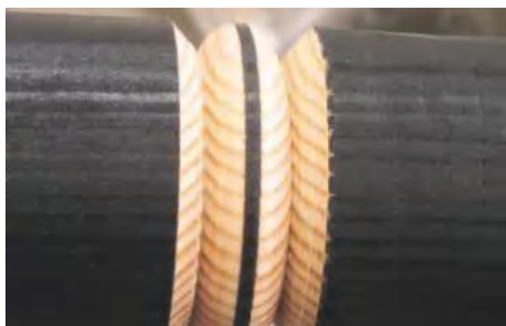
▲ Pic.19 The perfect bead. The black line at the top shows that I haven't changed the diameter. A bead should look as if the wood has been parted and the beaded inserted
